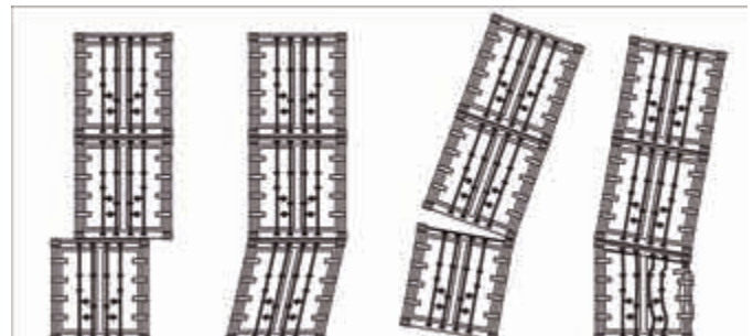
Container failure modes (from left) shear, racking, uplift, buckling.
