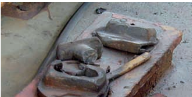
Base twist locks broken due to excess uplift.
