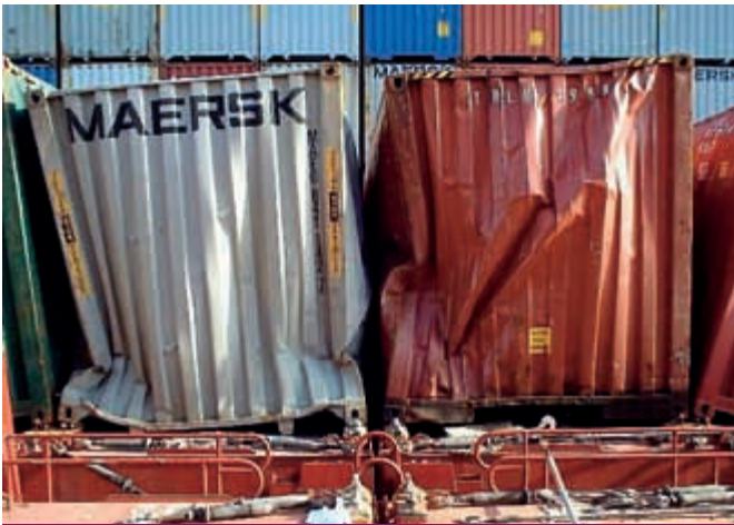
Buckled container corner post due to compression force.
