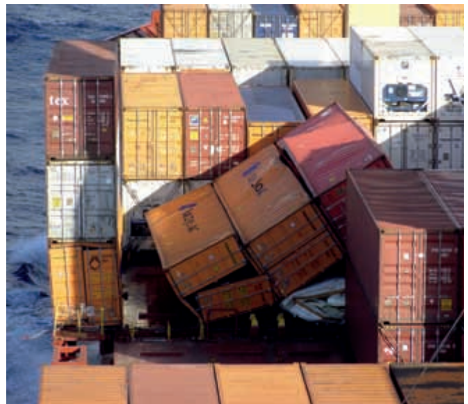
Racked container (bottom left) and toppled stack (centre) due to uplift.
